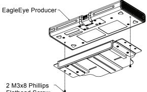
Flathead Screw (supplied with EagleEye Producer Universal Camera Mount Kit)
