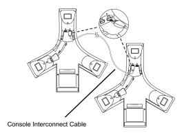
Using the 10-pin network cable included your Multi-Interface Module, connect another SoundStation IP 7000 into the SoundStation IP 7000 port, which is located on the back of the Multi-Interface Module.
