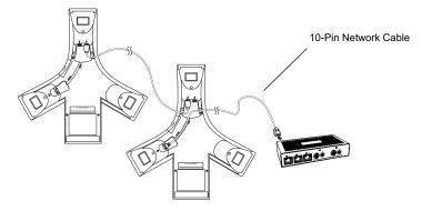
3. Using an Ethernet cable, connect a LAN port, located on the front of the Multi-Interface Module, to your local network port.
