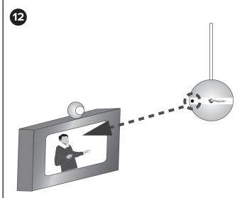
Point the dot (located on the band around the middle of the microphone ball) toward the main display.
