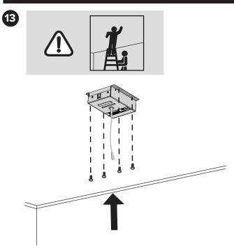
To attach the electronics enclosure, use suitable hardware for your ceiling type. Align the enclosure so that, when the Microphone Array is attached, the dot on the Microphone Array points toward the main display, as shown in Step 16.
