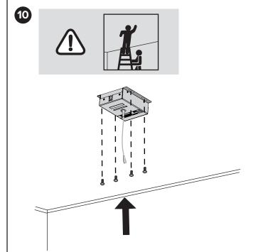
To attach the electronics enclosure, use suitable hardware for your ceiling type. Align the enclosure so that, when the Microphone Array is attached, the dot on the Microphone Array points toward the main display, as shown in Step 12 on this page.
