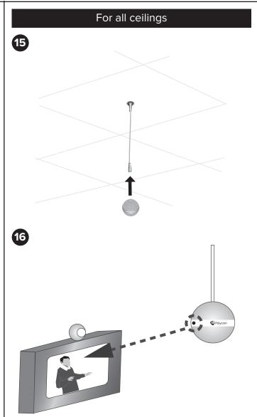
Point the dot (located on the band around the middle of the microphone ball) toward the main display.
