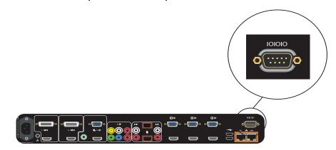
Use a DB-9 to DB-9 cable such as the Straight-Through Cable to connect to the RS-232 interface. The pinouts for this type of cable are listed in the following table:
