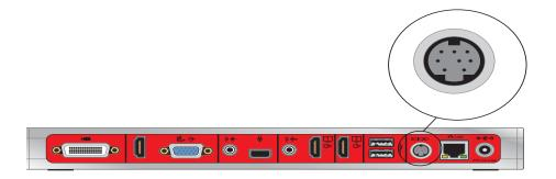
Use an 8-pin mini-DIN to DB-9 cable such as the Polycom RealPresence Group Series Serial Cable to connect to the RS-232 interface. The pinouts for this type of cable are listed in the following table:
