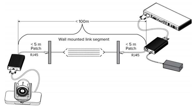
**Cable Bundling** Polycom EagleEye Digital Extender is based on HDBaseT technology, which limits how many data cables can be bundled together. The following table shows the maximum number of data cables permitted in a bundle.
